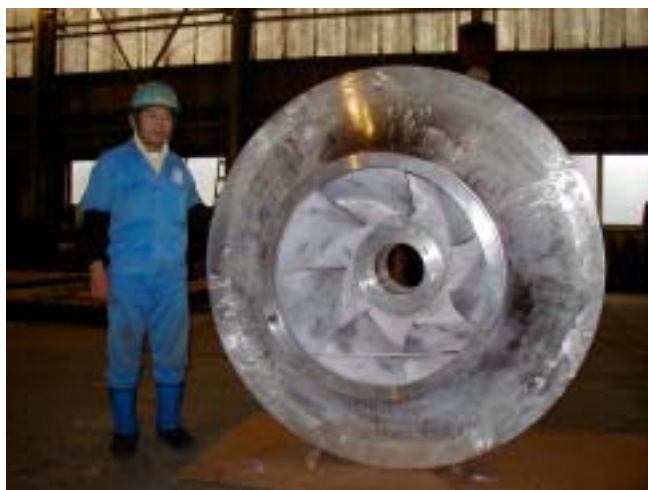
Impeller ( 1,700 860H) Super Duplex Stainless Steel (PI value 40) weight : 2,000Kg customer : Hitachi Industries
